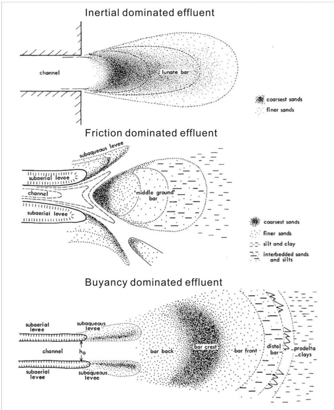
Figure 1 Three river-mouth depositional patterns in three different effluent conditions (From Wright, 1977)
