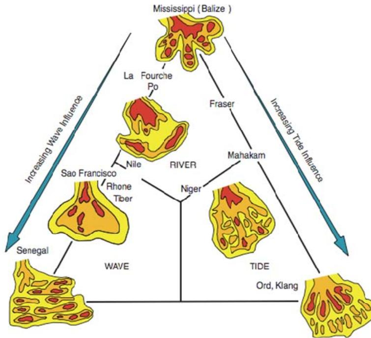
Figure 2 Depositional patterns under the interaction of river, wave and tide (From Bhattacharya and Walker, 1992 modified after Coleman and Wright, 1975)
