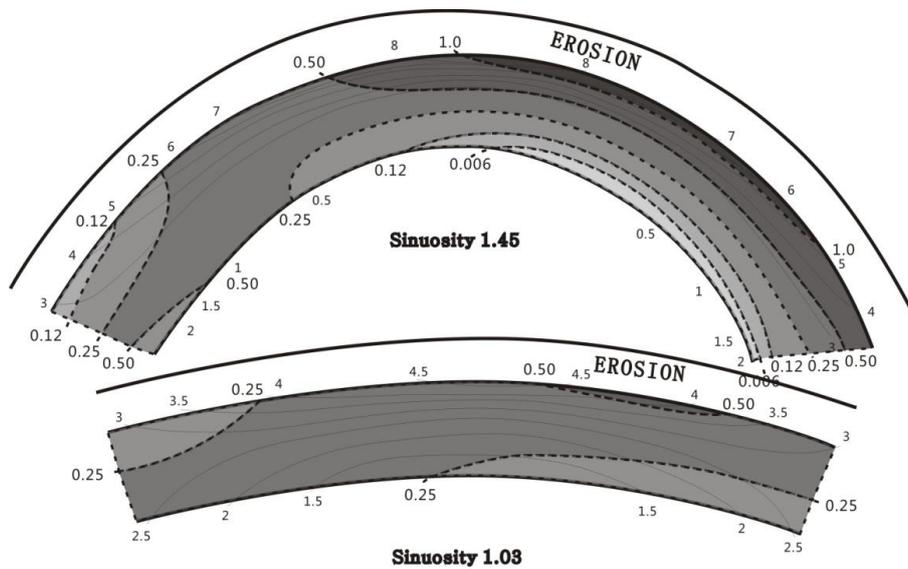
**Figure. 1** Two simulated point bars with different sinuosities. The channels have the same discharge, mean centerline depth, width and down valley slope. Solid contours display depth in meters and dashed lines display grain size in millimeters, revised from (Willis, 1989).
