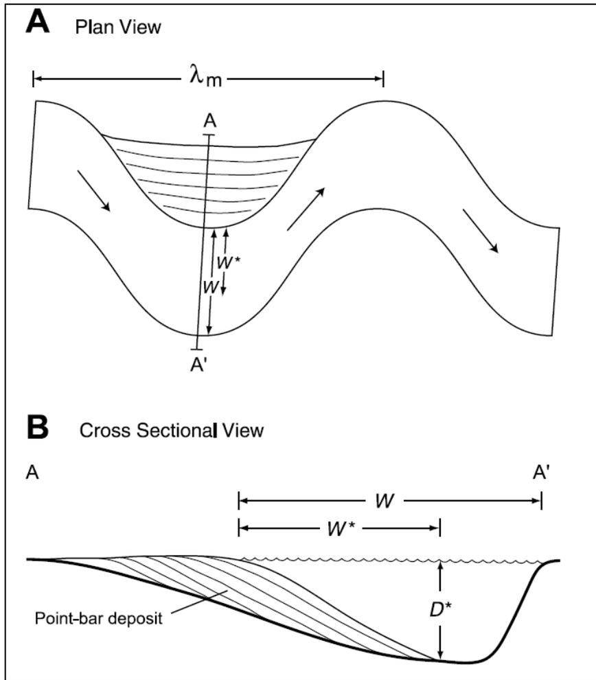
**Figure. 13** Schematic illustration of a meander bend in (A) plan view and (B) cross sectional view. Geomorphic parameters include bankfull channel width ( $W$ ) and meander wavelength ( $\lambda_m$ ). Bankfull channel depth and width are estimated from point-bar deposits in outcrop using the point-bar thickness ( $D^*$ ) and horizontal length of lateral-accretion surfaces ( $W^*$ ). Based on Lorenz et al. (1985).
