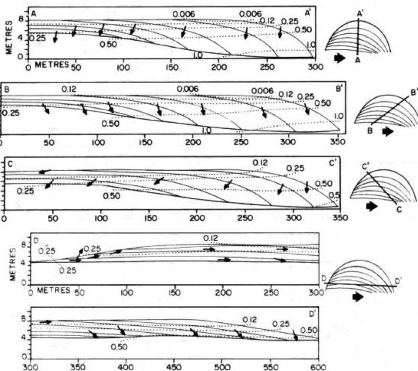
**Figure. 2** Cross-sections of simulated point bar deposit formed by down-valley translation and channel-bend expansion (Willis, 1989).
